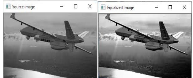
Fig. 6. The result of the alignment of the gray-scale image histogram
